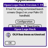
To activate OLH tap the **Activate**—button. To deactivate tap the **Deactivate**—button. If your device is performs a soft reset, OLH asks automatically for reactivation.
